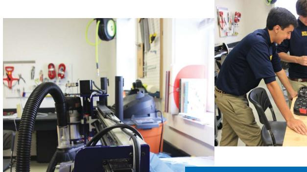
At left, the lab's Shopbot Desktop CNC Router allows students to prototype their ideas quickly in a variety of materials.
